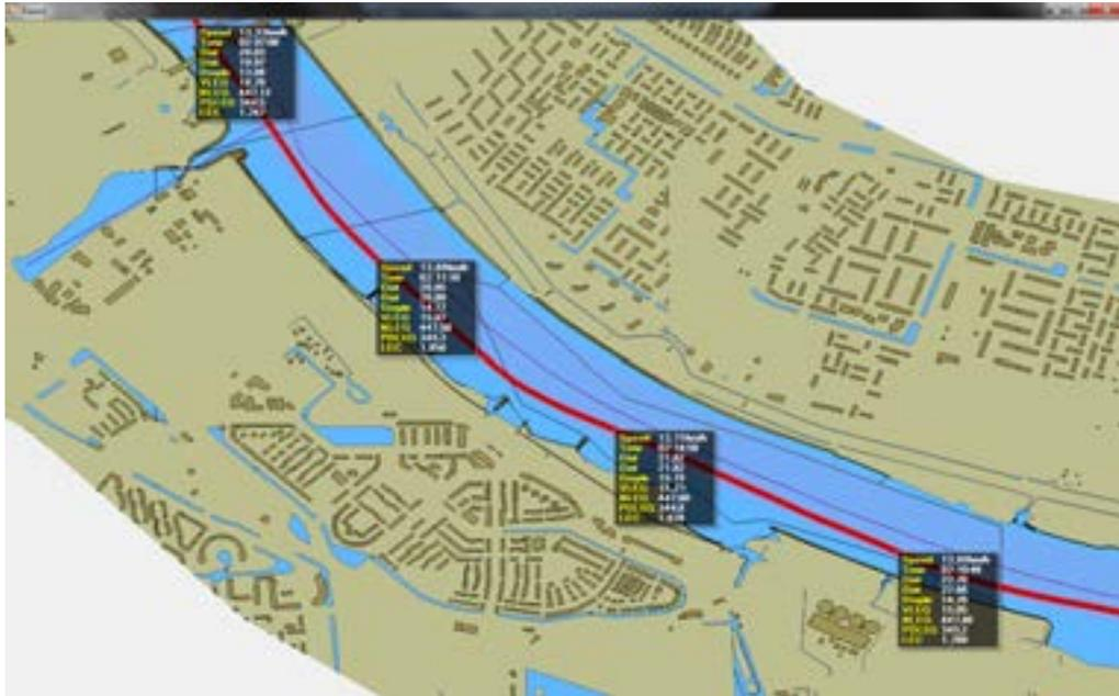
Figure 1: Optimal track presented on ECDIS, based on actual water depths
