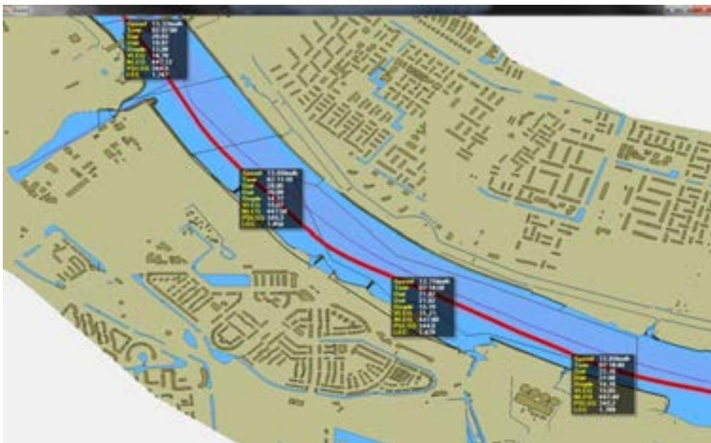
Figure 4: Optimal track presented on ECDIS, based on actual water depths
