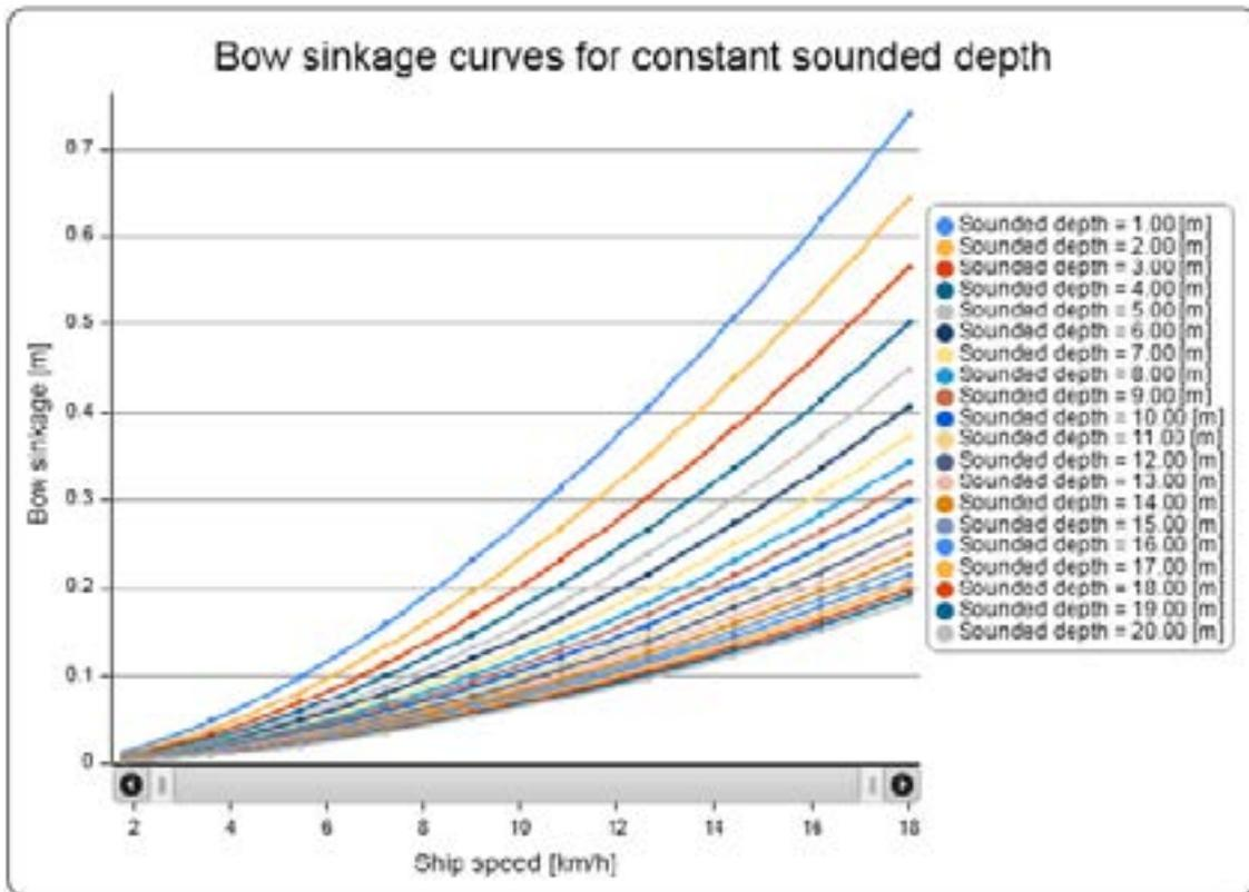
Figure 2: Bow sinkage for constant sounded depth
