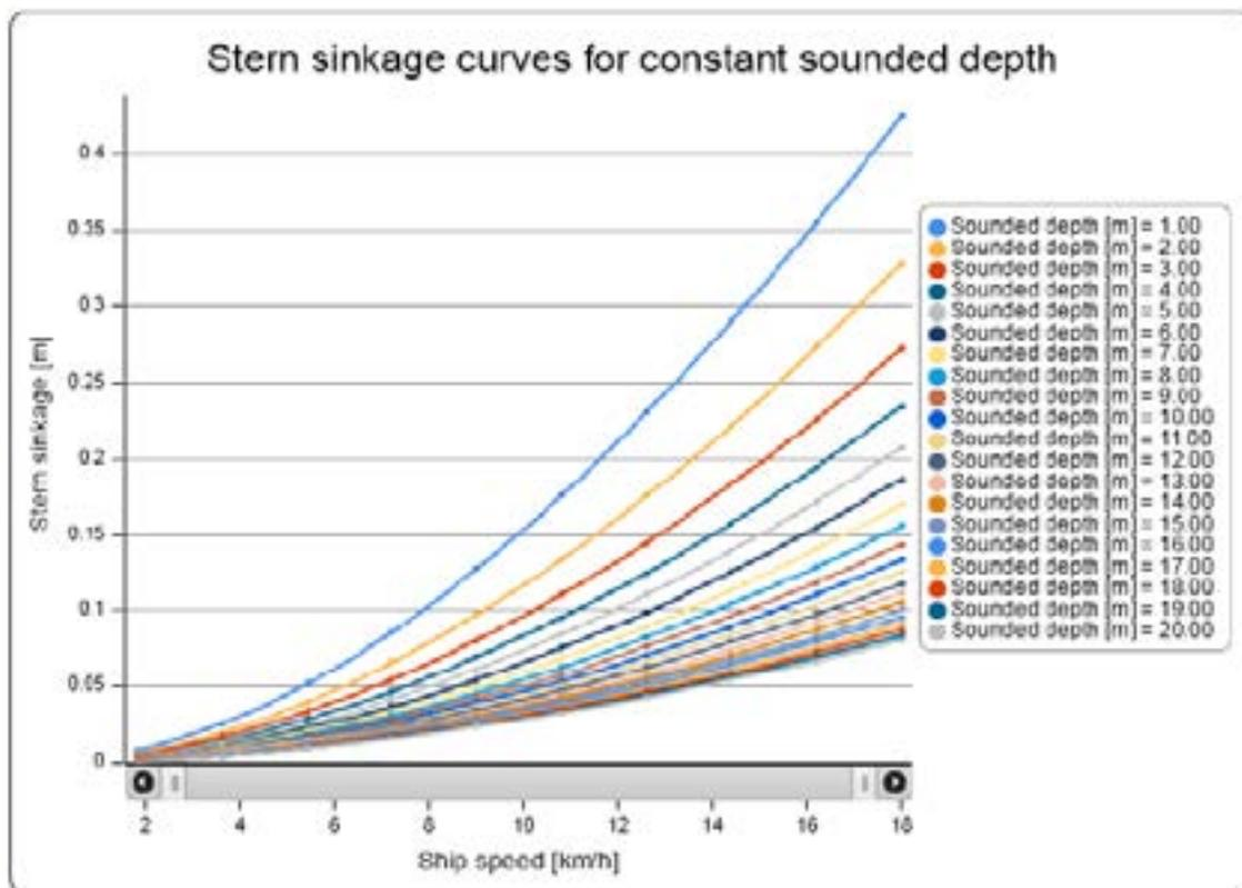
Figure 1: Stern sinkage curves for constant sounded depth
