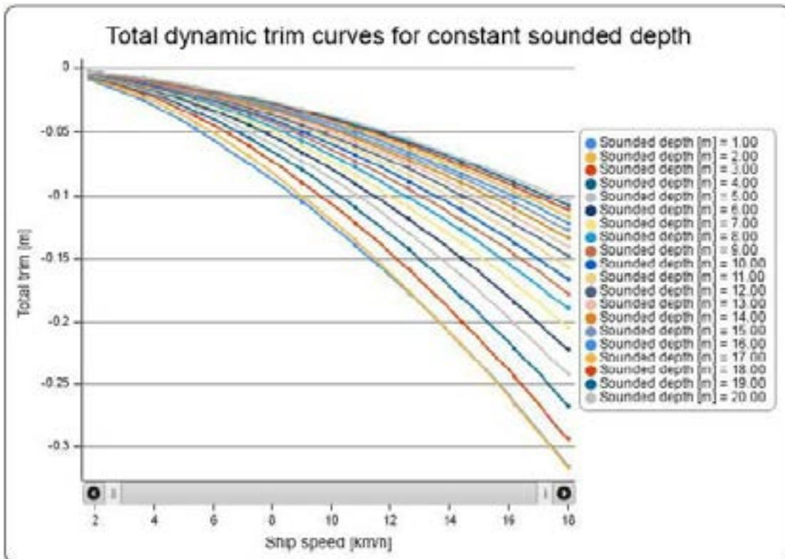
Figure 3: Total dynamic trim curves for constant sounded depth
