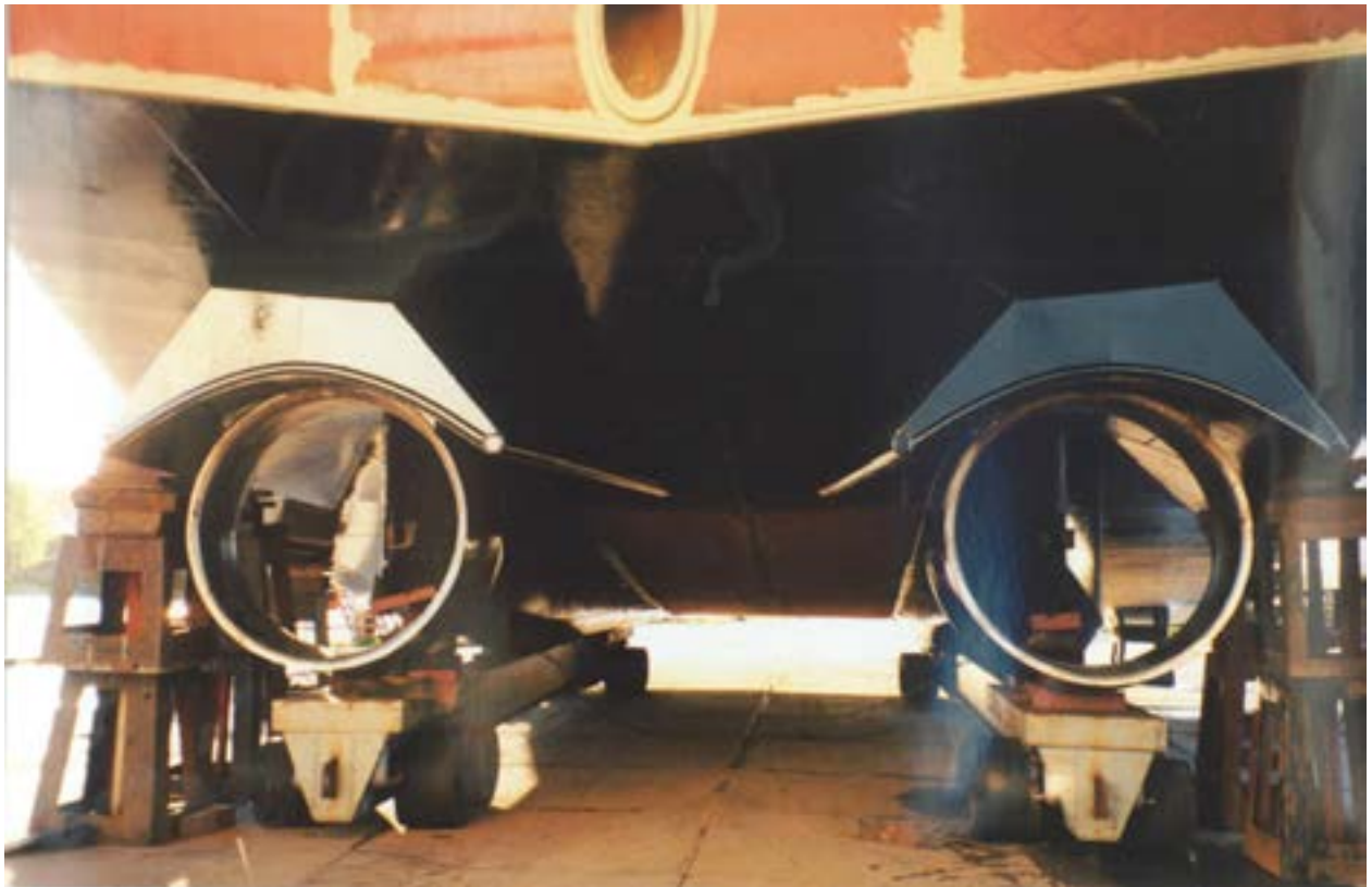
Figure 12 – Rear view on the existing fixed tunnels
